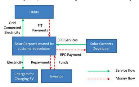
1.9.4. Solar PV, Battery energy storage, electric vehicles in virtual power plant model in a grid/minigrid/microgrid application owned and operated by utility, private sector, OEM
